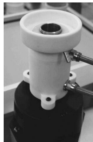
Fig. 4 New high-power cup-horn reactor (cavitating tube).
